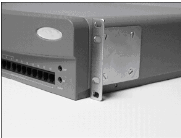
Figure 1 – Rack Mount Bracket Installation
