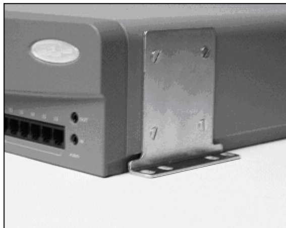
Figure 2 – Wall Mount Bracket Installation
